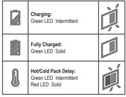
**Note:** The compatible charger(s) will not charge a faulty battery pack. The charger will indicate a faulty battery pack by refusing to light.
